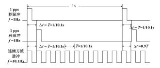
图 5 秒脉冲与秒脉冲或连续方波脉冲的时间间隔规律图 Fig. 5 Plot of time interval pattern of second pulse vs. second pulse or continuous square wave pulse
